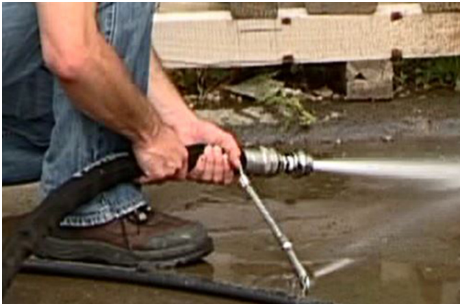
Fig. 3: Flushing the Discharge Hose
